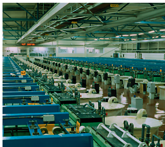
The phase-out of mercury cells for the production of chlorine (photo) is well underway, but OSPAR's 2010 target for full phase-out is not achieved
